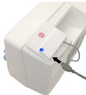
Figure 10.1.6. connecting the PhysioFlow Q-Link.
